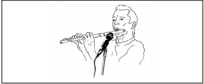
Fig. 9: Microphone placement for the flute.
